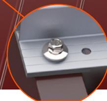
Installing the Quick RAIL mounting structure produces no swarf thanks to our special screws that create their own extended thread. Why is this important? With stepping on swarf during installation, micro-cracks occur in your roof structure. The damage is not visible right away, but certainly with time it has a major negative effect on the roofing properties.
